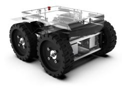
Excellent Performance and Precise Control 50KG Loading Capacity, 20° Climbing Capacity, Ramp Parking Mode
